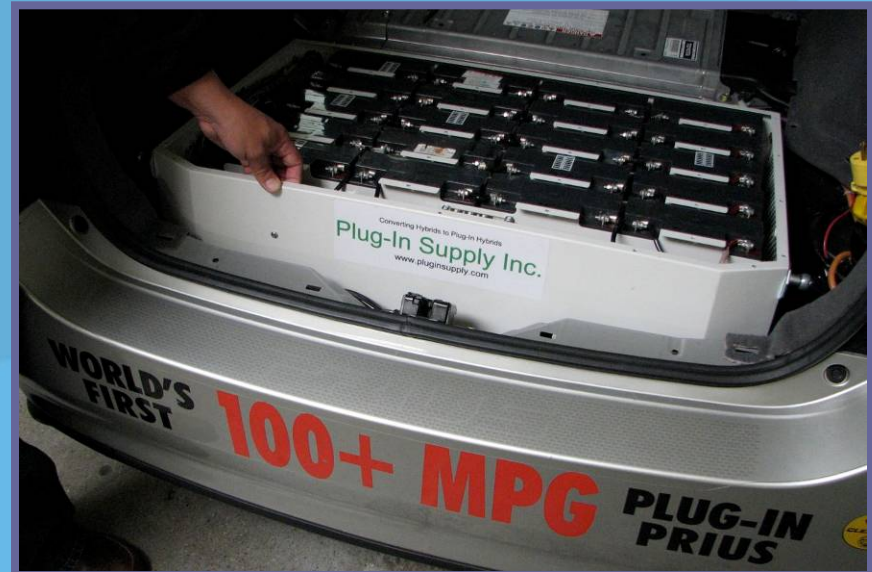
Left: nano-phosphate lithium (A123Systems) Above: lead-acid (EAA-PHEV/Plug In Supply)
