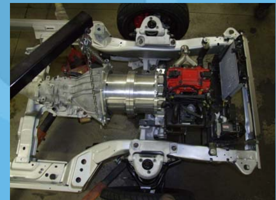
Gen 2 Series PHEV Powertrain in a running rolling chassis
