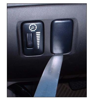
11) Remove the left side vent piece and plug covering the hole next to the dimmer switch.
