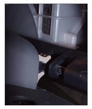
You may also need to unclip the little hydraulic piston that keeps the door from falling open too quickly. Next, grasp the bottom of the silver vent piece next to the glove box. Pull it toward you firmly. It should unclip at the bottom first. Then pull the whole unit straight out.
