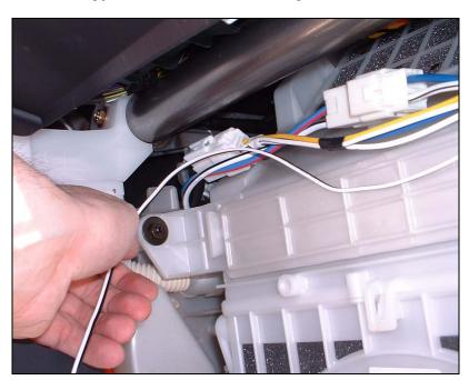
10) Thread the remainder of your wire through the hole where you had the plug out. You'll see another bundle or two of wires running just above and behind the lower glove box area.
