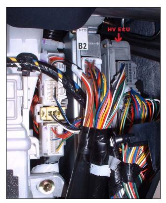
You'll probably need to carefully push some of the bundles of wires out of the way and carefully wedge your hand into the space. Reach in and release the catch on the lower-most gray plug of the HV ECU (H14).
