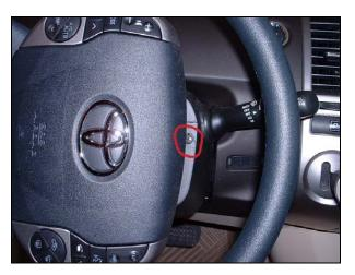
Then turn the wheel 180 degrees left (90 degrees from normal position) and remove the black screw on the left side of the steering column.
