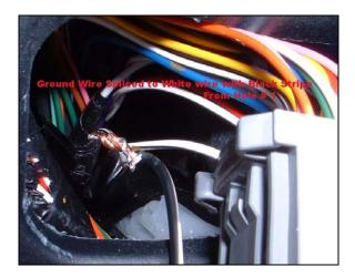
If you have a splicing connector that would work very well here as well. If you do cut the wire to splice into it, be sure to solder and tape the wires together to make them secure.
