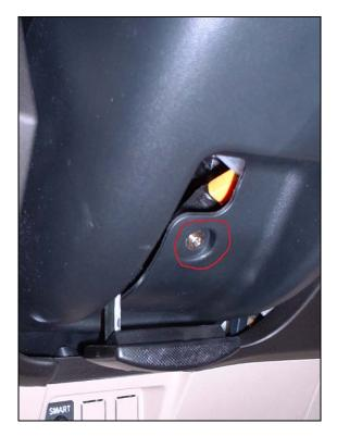
Then, turn the steering wheel 90 degrees right and remove the black screw that becomes visible on the right side of the steering column.
