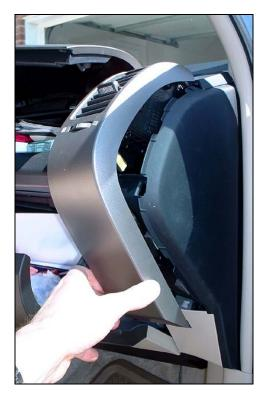
You'll eventually need to remove the driver's side (far left) vent piece as well. Finally, remove the smaller square plastic piece just below the passenger side vent--it pulls straight out.
