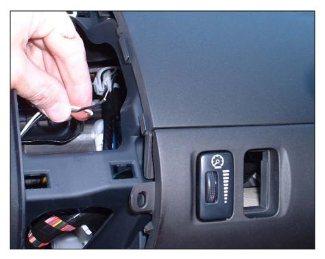
Once located, thread it up along the far left side over to the opening next to the dimmer switch. You'll need to remove the wire from the coat hanger to get it through that hole. Pull all the excess wire out of the hole in the dash where the button will go next to the dimmer switch.
