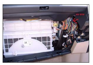
There are 3 vertically oriented ECUs, 2 with white. The HV ECU is the one farthest to the right and is the only one with gray plugs.
