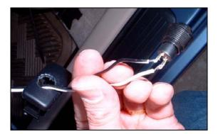
You may not be able to get the nut flush due to the residual fins, but it doesn't matter as long as the button is secure. Now solder the wires to the connectors on the button. DON'T overheat the connectors, as it could damage the button's internal contacts. (It doesn't matter which wire goes onto which contact.)
