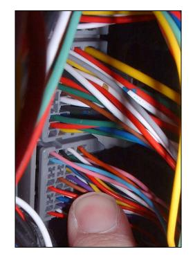
There's a small catch on the right side of the plug that you need to squeeze in to get the plug out. Remember the orientation of the plug so you can properly identify the holes where you need to insert the connector pin and wire. Once removed pull it carefully through the lower most opening (where you removed the square plastic piece below the vent piece).
