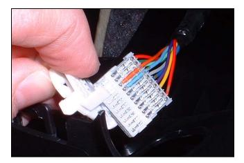
You should remove between 1 and 3 of those pins--2 is probably safe, 3 might be better, since if you plan to install an OEM button at some point, you'll probably need more pins for that. (You need one pin for the procedure, but it's handy to have a back-up.) To remove the pins, you can use your paper clip to start the process of sliding them out, and then they just pull right out.
