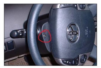
Carefully pull down on the lower portion of the steering column cover until it releases. Mine was a bit stiff/stuck to the upper part and you may need to carefully use a butter knife or screwdriver to start prying them apart.
