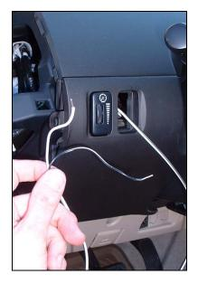
11) To attach the button to the plug, you'll need to trim off several of the 'fins' in the middle. I used wire cutters for most of that, then a box cutter to trim it down further.
