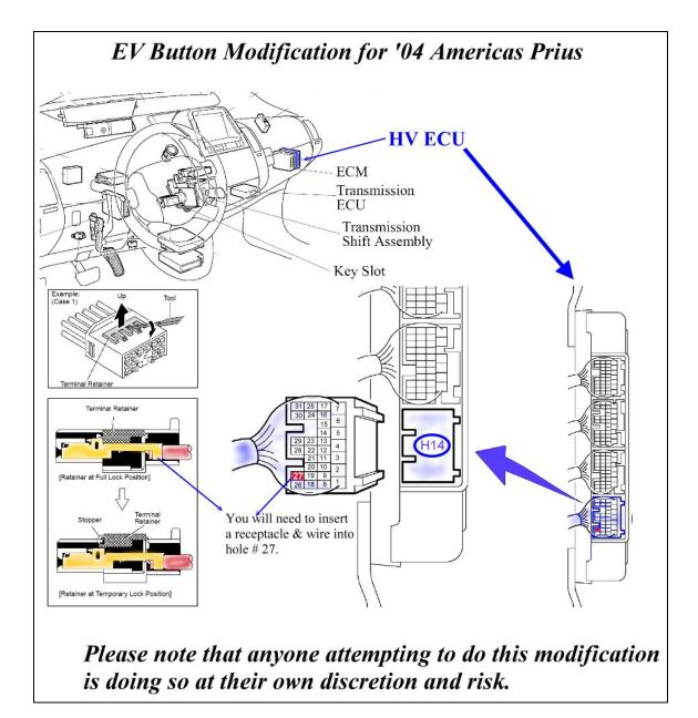
6) Locate the HV ECU just to the right of and a little behind where the glove box was.
