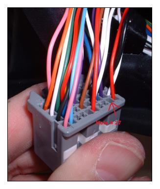
You will need to use the little jeweler's screwdriver on the end of the connector pin to push the pin all the way in. Once it's in, push the terminal retainer back down to lock the pin into place.
