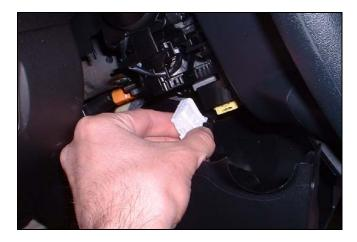
3) 2 little clips keep a cover locked in place. Pull those apart and remove the cover. Inside you'll see lines of silver connector pins--some with wires attached, some without.
