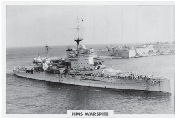
The HMS Warspite: Commissioned in 1913, it was the first warship to use only oil fuel, the first to mount 15-inch guns and the first to reach a speed of 25 knots.
