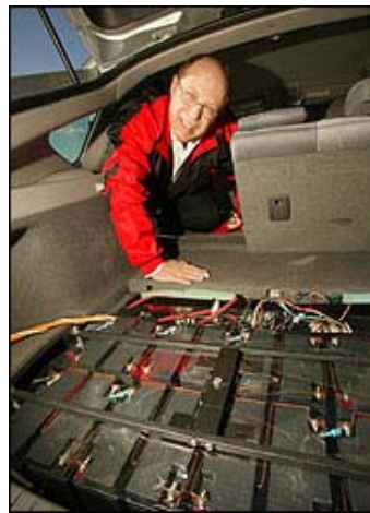
Andrew Sacks for The New York Times Ron Gremban modified a Toyota Prius by installing auxiliary batteries.
